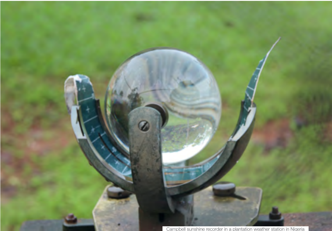
Campbell sunshine recorder in a plantation weather station in Nigeria
